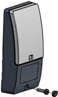
Figure 4: Removal of escutcheon
